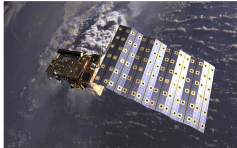
Figure 1: Illustration of the MetOp-SG A spacecraft carrying the Sentinel-5/UVNS instrument.
